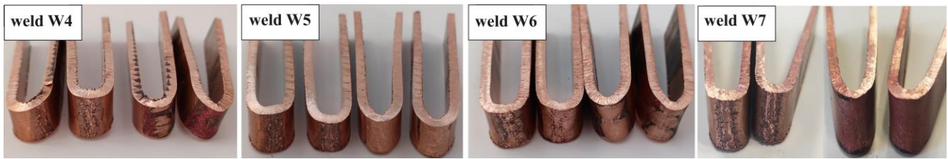
Figure 6. Specimens sectioned from welds W4 – W7 after transverse bend test.
